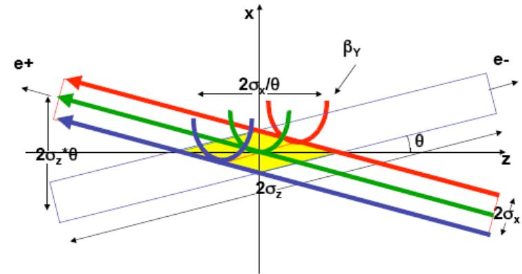
New collision scheme (tested with the **SIDDHARTA** experiment)
